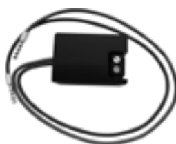
Pre-Load Electronic Assembly 760-12 Improves pre-load capability to at least 300N for DC operation. A short buzzing sound is audible in the electric strike for about 0.5 seconds. Continuous current-resistant, holding current is reduced. Compatible with standard effeff electric strikes
